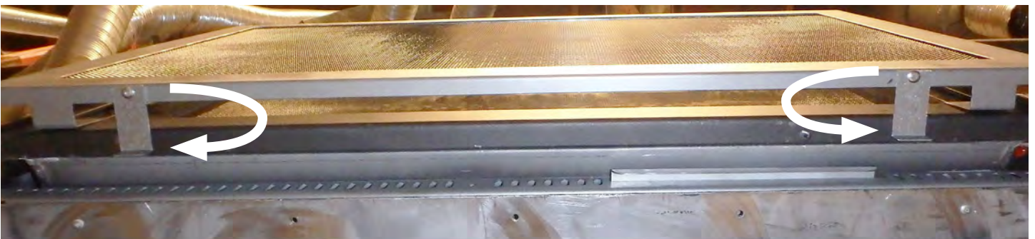
Figure 13.4.04: Rotate the retainer tabs under the door frame to secure the screen in place.
