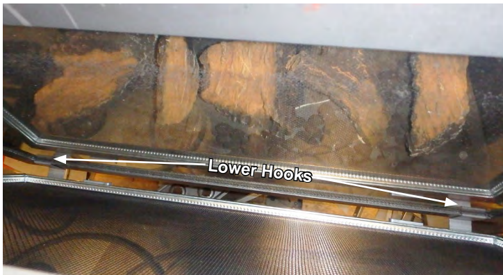
Figure 13.4.02: Insert the hooks in the bottom of the screen between the door frame and glass. At the same time insert the hooks in the top of the screen into the holes at the top of the door frame.
